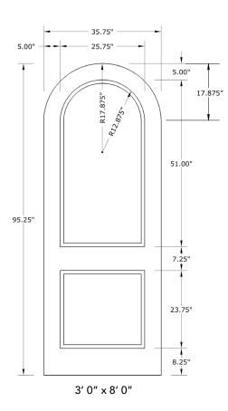
NOTE: BY REQUEST, DOOR HEIGHT COMES IN VARYING DIMENSIONS TO A MINIMUM OF 95". EXCESS WILL BE TAKEN FROM BOTTOM RAIL. ALL OTHER DIMENSIONS WILL REMAIN THE SAME.
